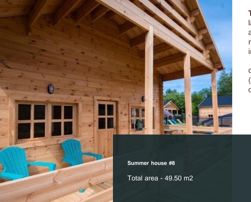
The kit includes: wall beam single-layer (135hx44), a set of hardware, additional elements, floor beams, racks, sheathing "lumber imitation", terrace board, rafter system (rafters, crate,), floor arrangement (floor board, logs), window and door blocks.
