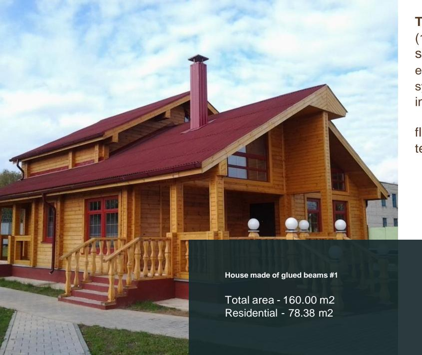
The kit includes: wall beam (140hx210), beams floors, set hardware, additional elements (elements rafter systems (rafters, crate, insulation, screeds, overlays),
